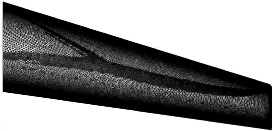
a) Fine surface grid, TAU adapted
